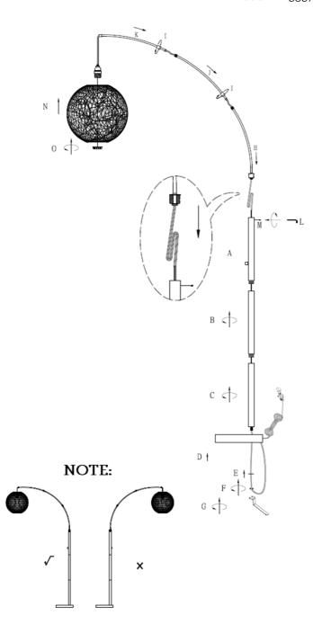
Please begin assembly by laying all parts down on the ground. The arms are easiest to assemble if you assemble them first, before they are attached to the lamp body.
